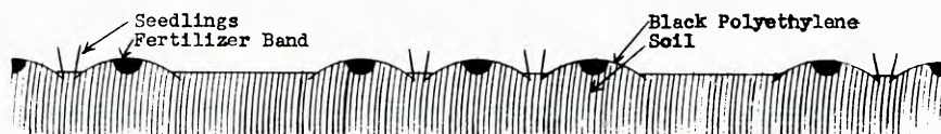
Fig. 30. Profile showing position of seedlings, fertilizer band and black polyethylene film. Single row method.
